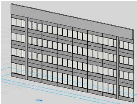
This is a stucco panel system within a curtain wall system. The glazing on the ends is butt joint, while the interior section glazing is exposed mullions. The two 24" square columns are to stay 15 feet from each end regardless of the length of the curtain wall. The top portion is an 8' tall parapet that extends 18 inches from the centerline of the curtain wall out. The system should grow or shrink floors easily.
