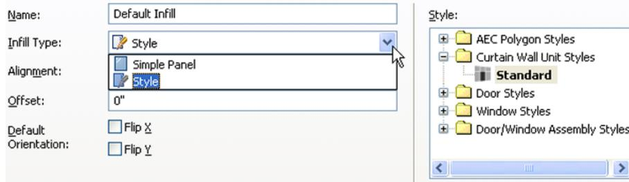
Infills can be either a simple panel or a style definition. A simple panel is just that a solid infill with a specified offset and thickness
