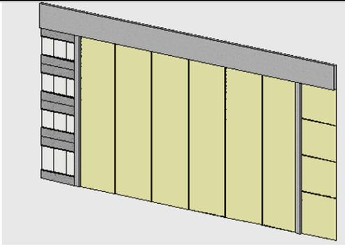
OK back to the drawing and your curtain wall should now have a left side completed with butt jointed glass and stucco panels
